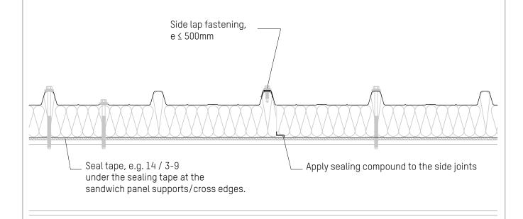
Roof panel - Fire safety, sound dampening and thermal insulation
