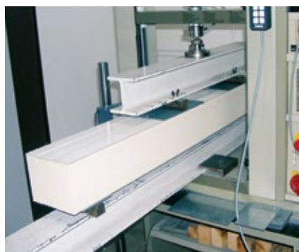
Computer-aided quality checks: bending test
